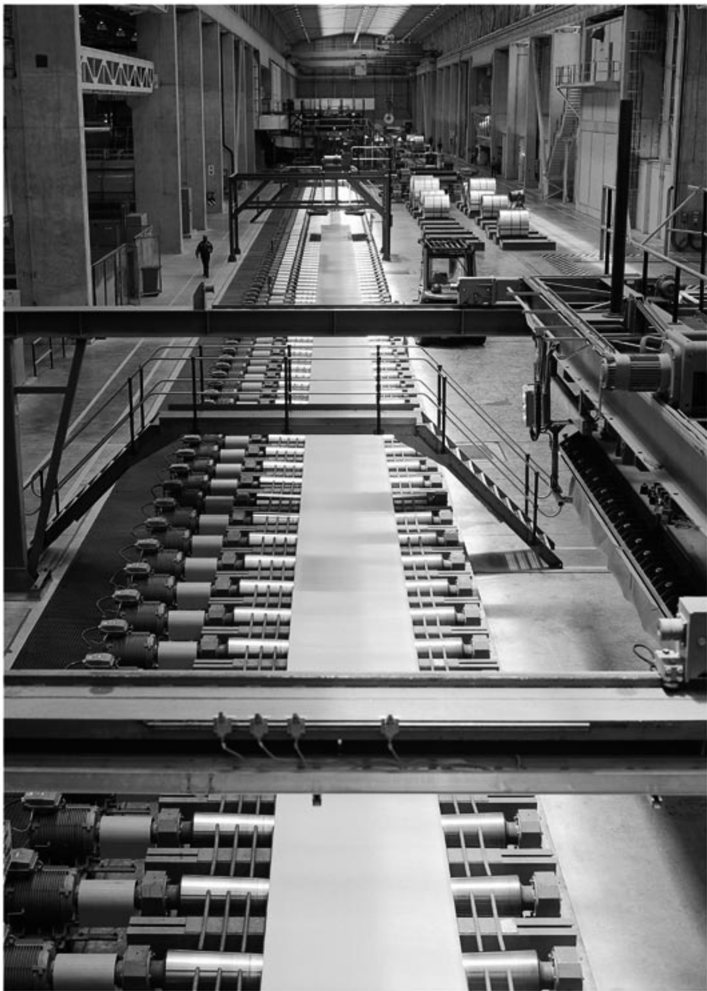
Hulett Aluminium's new R800 million hot line which is now in start-up phase, has the highest level of automation including artificial intelligence applications in the programming of process control software.
